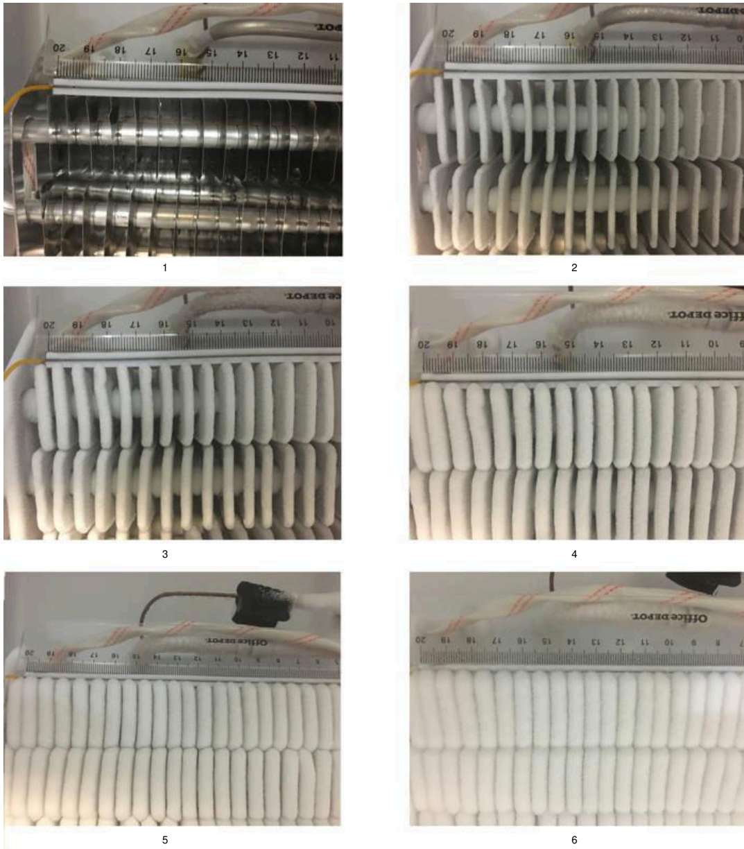
Figure 5. Frost Formation Process
