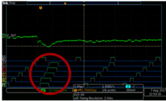
Figure 7. Phase-Management Comparison During Load Step
