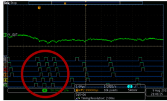
Figure 7. Phase-Management Comparison During Load Step
