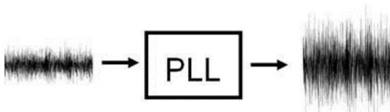
Figure 1. Input Reference Noise is also multiplied by the PLL
