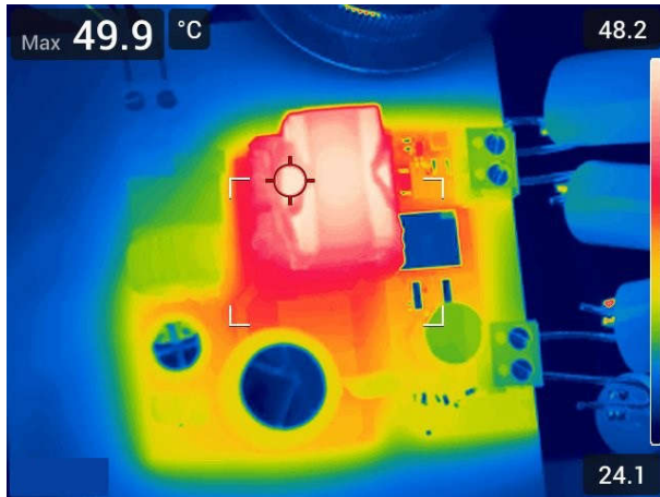
Figure 2-5. PMP23331 Thermal Image, 230-Vac Input, Top Side
