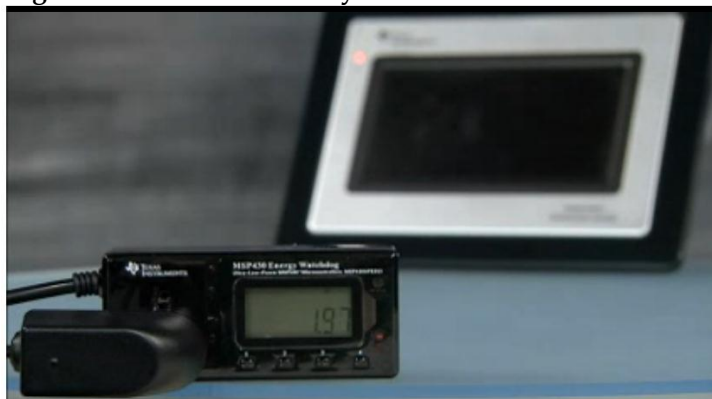
Digital Photo Frame Standby Mode = 1.97 Watts
