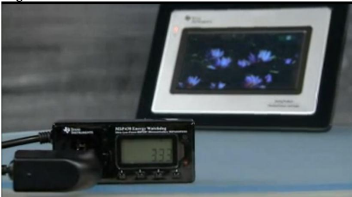
Digital Photo Frame Active Mode = 3.33 Watts
