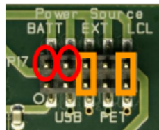
Figure 5. Power Selection Jumpers of TRXEB
