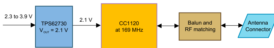
Figure 3. Block Diagram of wM-Bus RF Subsystem at 169 MHz
