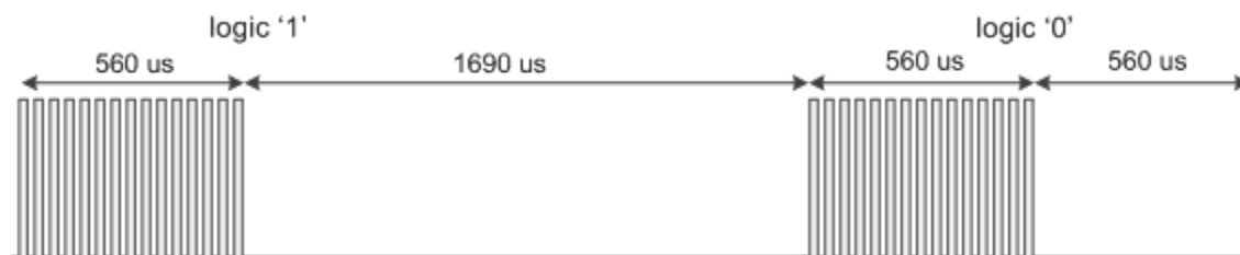
Figure 4. Pulse Distance Protocol, Bit Encoding
