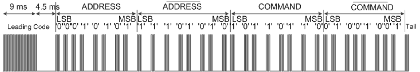
Figure 5. Pulse Distance Protocol, Data Frame Format
