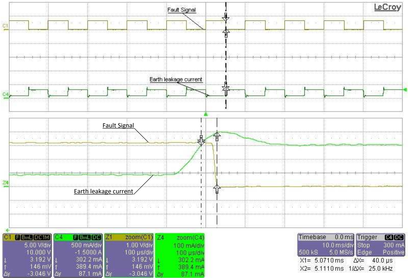
Figure 23. Response Time to GND Fault
