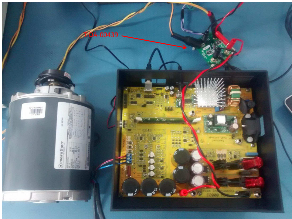
Figure 26. TIDA-00439 Connected to C2000 Motor Control Kit
