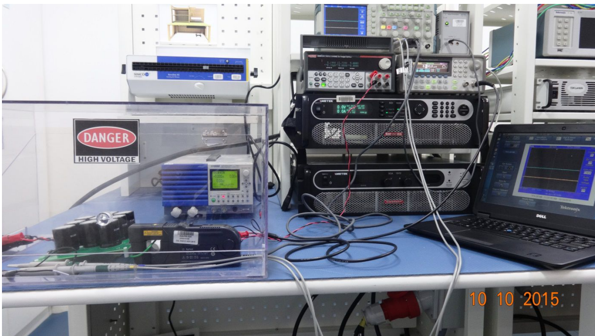
Figure 75. Miller Clamp and Desaturation Detection Test Setup
