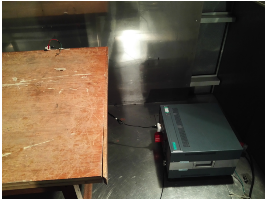
Figure 21. Conducted Emission Test Setup
