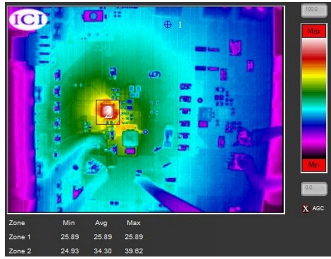
Figure 5. bq25890 With I_{CHARGE} = 2.25 A and bq25898C Disabled
