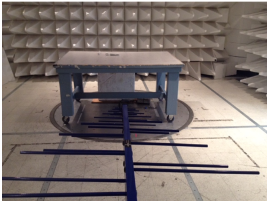
Figure 43. EMI Setup for CISPR22 Emissions Testing
