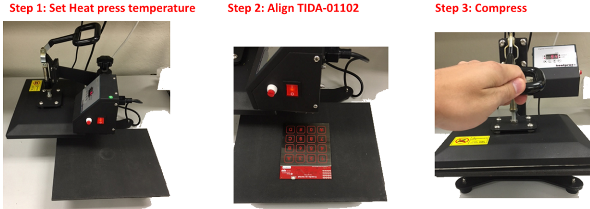
Figure 31. Example Compression Technique Using Heat Press
