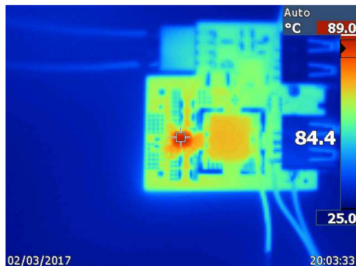
Figure 4. Thermal Image at Full Load
