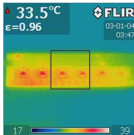
Figure 11. Thermal Image of Tail-Light Function at 25°C, 12-V Input Voltage
