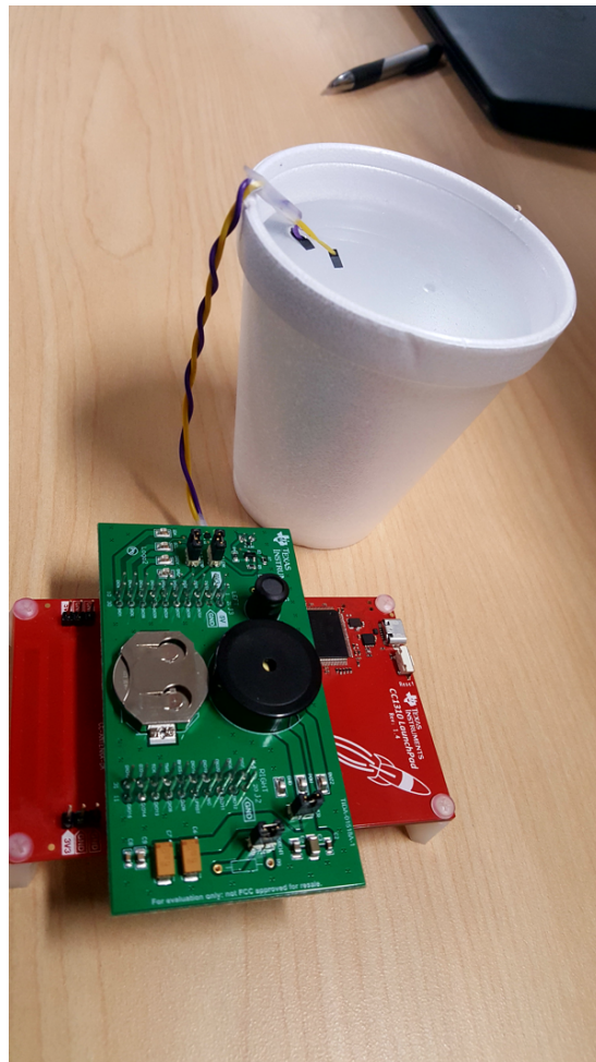
Figure 23. Test Setup of Water Leak Detection
