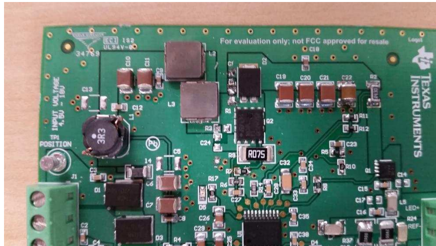
Figure 27. TIDA-01581 With Unshielded Inductors (Vishay IHLP-2525BD-A1)
