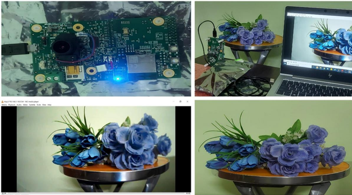
Figure 3-22. Video Streaming- Camera Module (Top Left), Camera Video Streaming Subject (Top Right), Camera Video Streaming on VLC (Bottom Left), Subject (Bottom Right)
